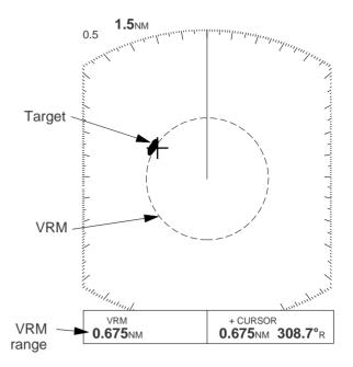
Figure 2-8 Measuring range by the VRM
